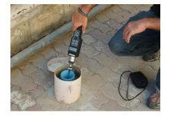
PhoCheck+ was used to demonstrate that there were no soil contaminants coming from leaks in the underground tanks at fuel stations, a mandatory requirement by the Israeli Environmental Protection Agency.
